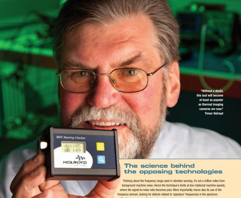
Essentially, Holroyd's MHC (machine health checker) comprises a 'smart' sensor with signal processing, battery and display all in a small magnetic instrument. Technicians simply attach it, in any orientation and location, to the machine in question, press the button and around 10 seconds later they see readings of wear-related surface and sub-surface 'distress' and dB (noise level).
